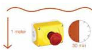
IP67: Submersion to one meter for 30 minutes
